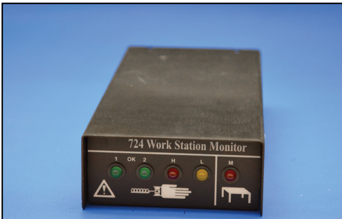
Figure 11. SCS 724 Workstation Monitor mounted on benchtop.
