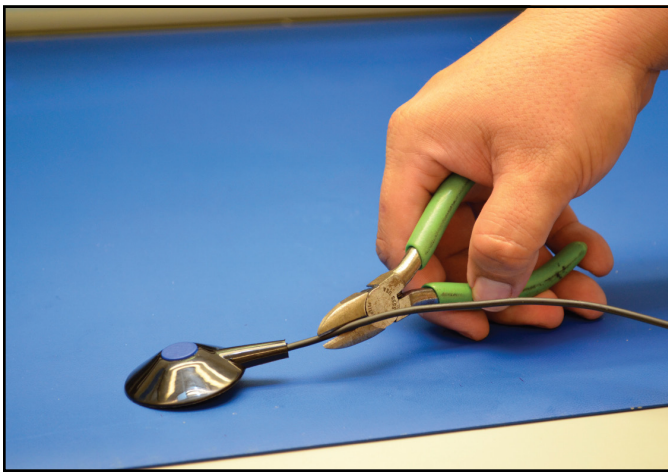
Figure 7. Cutting off table mat ground snap.
